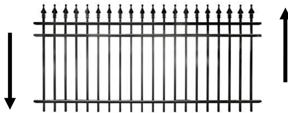
Racking a Panel
