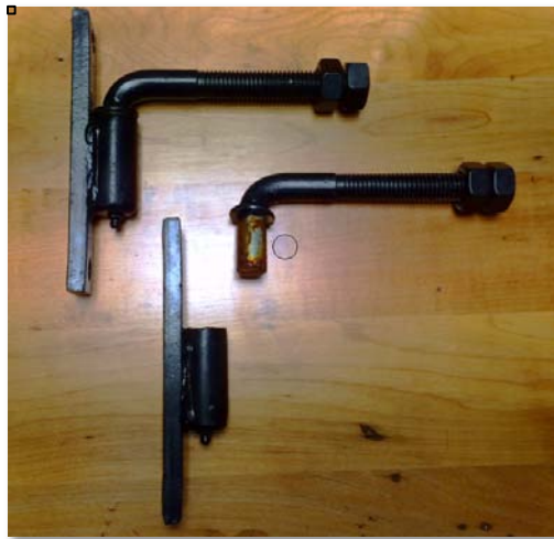
Figure 20 - The J-Bolts Will Separate at the Swivel Point
