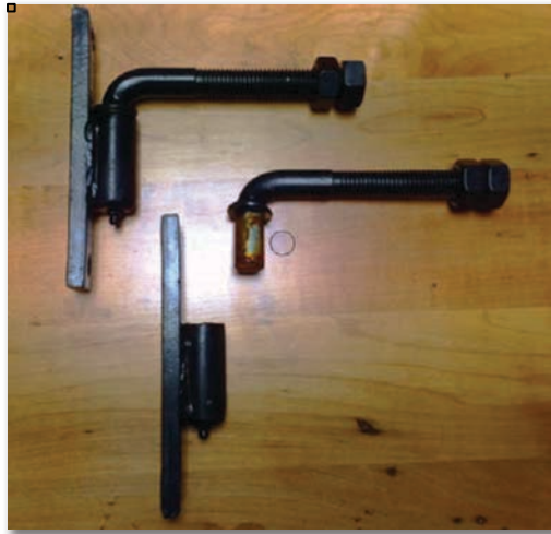
Figure 16 - The J-Bolts Will Separate at the Swivel Point
