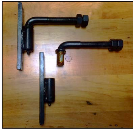
Figure 14 - The J-Bolts Will Separate at the Swivel Point
