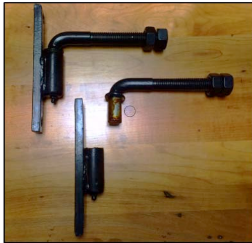
Figure 25 - The J-Bolts Will Separate at the Swivel Point
