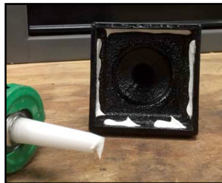
Figure. 21 - Apply Under the Cap
