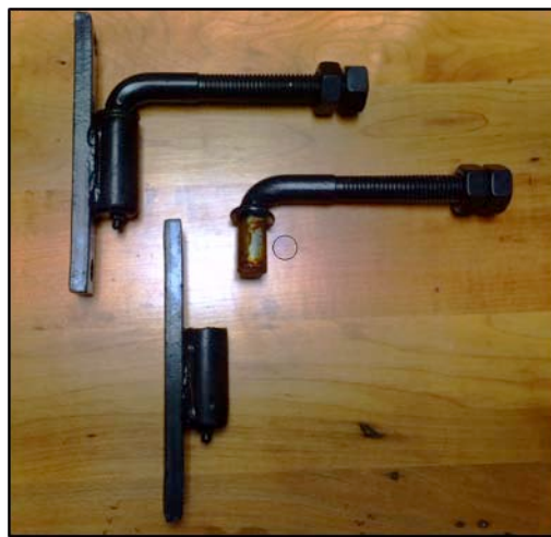
Figure 25 - The J-Bolts Will Separate at the Swivel Point
